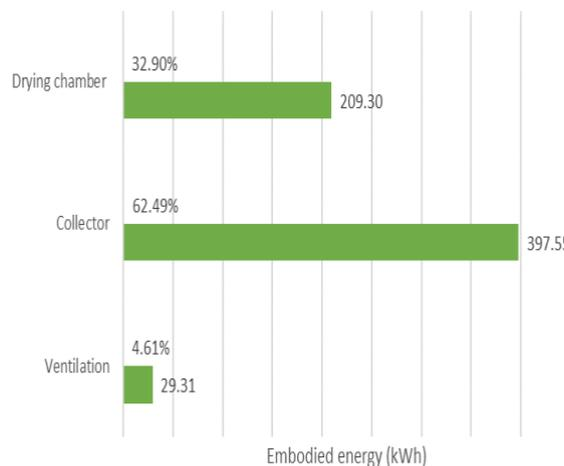
Figure 2. Embodied energy for each solar dryer unit component
