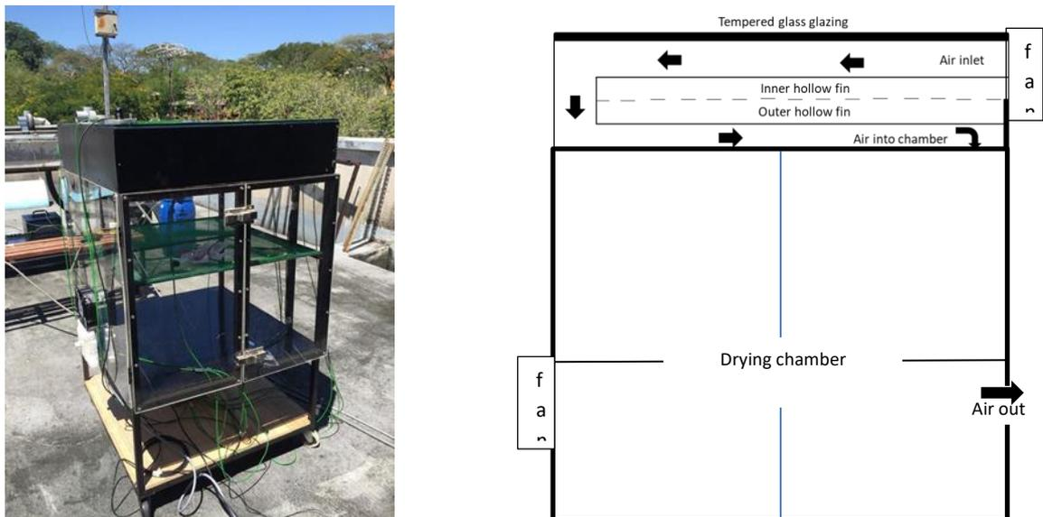
Figure 1. Solar collector mounted to the drying chamber in a greenhouse dryer; (a) photograph, (b) schematic
