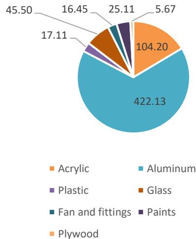
Figure 3. Break-up of embodied energy of different material used for construction of the solar dryer
