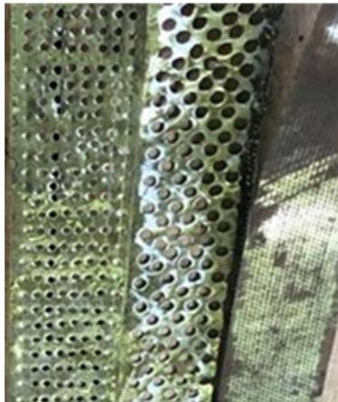
Figure 4. Sieve Size 3 mm, 5 mm and 10 mm
