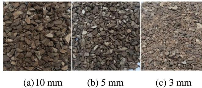
Figure 6. Coconut Shell Particle Size
