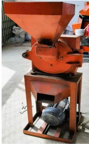
Figure 3. Grinding Machine
