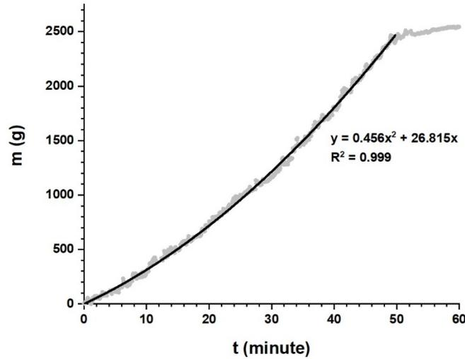
**Fig. 6.** Evaporation rate in the steam boiler
